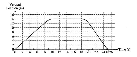
2. The vertical position of an elevator as a function of time is shown above.
